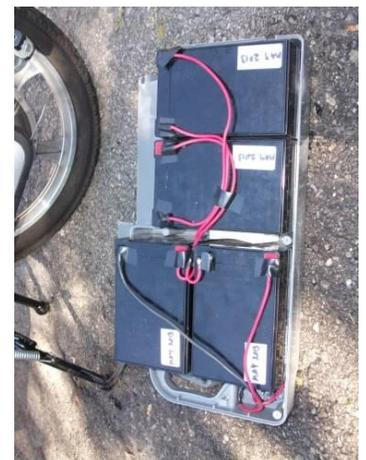
This E-Scooter battery pack consists of 4x12V, 10A/H batteries
